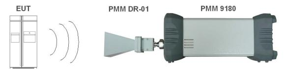
Fig. 3-3 Radiated emission test setup – PMM DR-01 Horizontally polarized with PMM 9180
