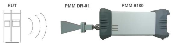
Fig. 3-1 Radiated emission test setup – PMM DR-01 Vertically polarized with PMM 9180
