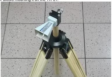
Fig. 2-2 PMM DR-01 with Antenna holder on the TR-01
